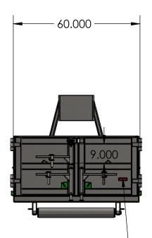
Weld serial no. on Back door & Floor-
